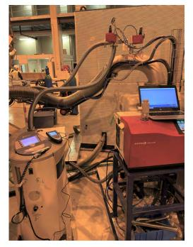
**Figure 6** Leak detector, on left side, and vacuum pumping system connected to PF5 cryostat.
