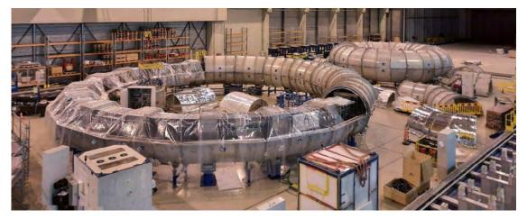
**Figure 2** The dedicated area for the cryostats: On the right, the smaller cryostat is assembled and cold testing of the PF6 coil is in progress. On the left, the medium sized cryostat is about to be assembled for the final cold test of PF5.
